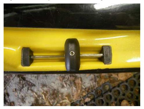
The wire is secured to the skeg with a 2mm allen grub screw.
