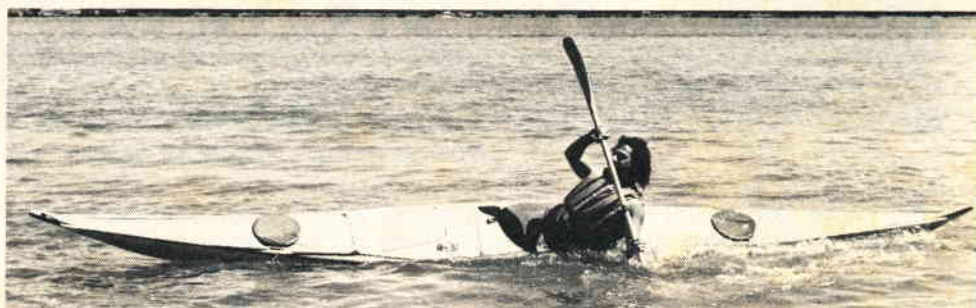
Nordkapp kayak. Note hatches which have canvas covers in this instance. For more boisterous conditions an aluminium or fibreglass hatch seals the hatch beneath the canvas covers. The paddler's spray sheet seals the boat completely and is an absolute necessity because of the very low freeboard of these craft
